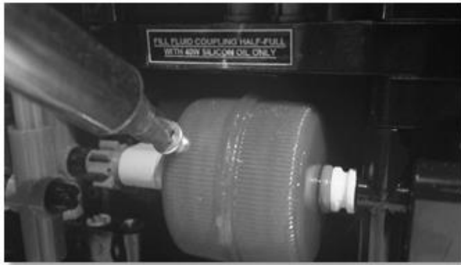
Figure 10: Removing Fluid Coupling Oil-Fill Screw
